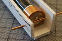
3. Take the sharp ends of the metal rods out of the protective foam. Careful, these ends are dangerous! Poke the sharp ends into the foamcore. These rods need to be in contact with the batteries, holding them snuggly together.
