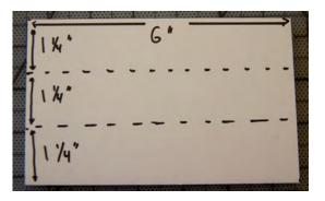
1. Read the safety notices! Then start by cutting out a piece of foamcore that is 6" by 3.75". Divide the short side into 3 even 1.25" segments
