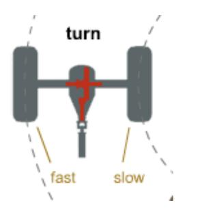
Drive wheels must be capable of rotating at different speeds
