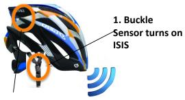
2. 3-axis accelerometer assembly detects impact
