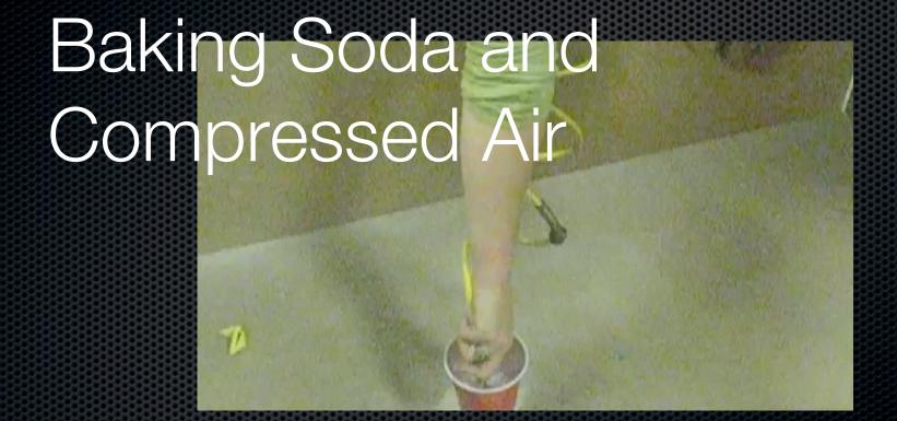
Compressed air directly into baking soda, material disperses well
