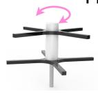
Agitators will loosen the flour in the canister, thus avoiding packing and reducing measurement variation.
