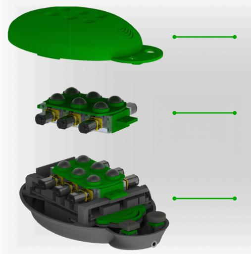
Letter Bug has been designed keeping robustness in mind by having every internal component mounted and fastened securely.
